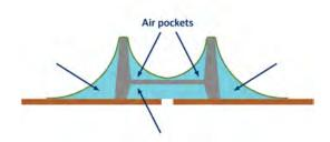
High sided tools will create large pockets of air that the vacuum pump or tank will need to remove.
