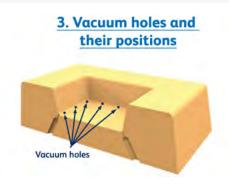
Vacuum holes or slots should be positioned at the lowest point in cavities or at changes in sections. Every corner requires a hole and they should generally be spaced 25mm (1") apart.
