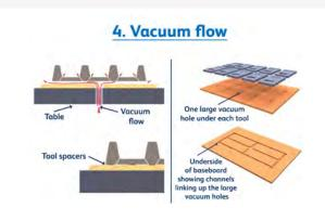
When using multiple tools, try to create an even vacuum flow from the main central vacuum hole on the table, to the underside of each of the tools.
